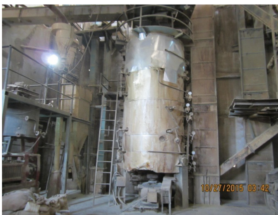
Steam heated soybean cooking pressure cooker
