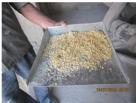
Crushed soybean with hulls
