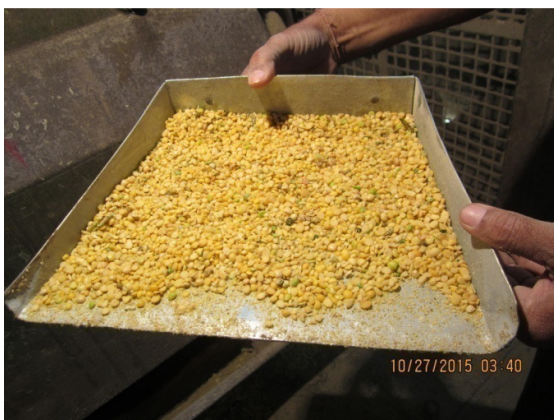
Broken soybean cleaned from hulls
